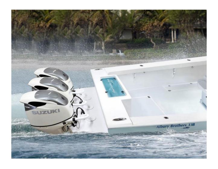
The 33B has a closed transom and Armstrong Bracket, which accommodates Triple Engines.
